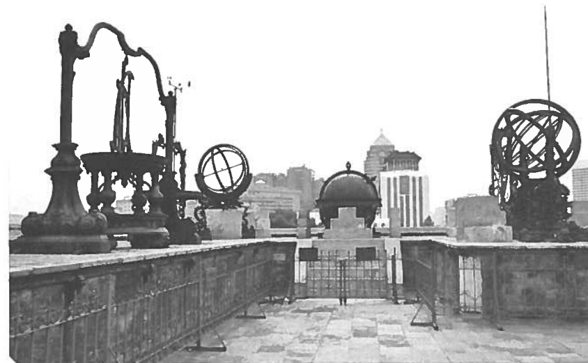
A 2009 photograph of the Beijing Ancient Observatory. Instruments from left to right are the azimuth theodolite (1715), altazimuth (1673), ecliptic armillary sphere (1673), celestial globe (1673), and "new" armillary sphere (1744).
