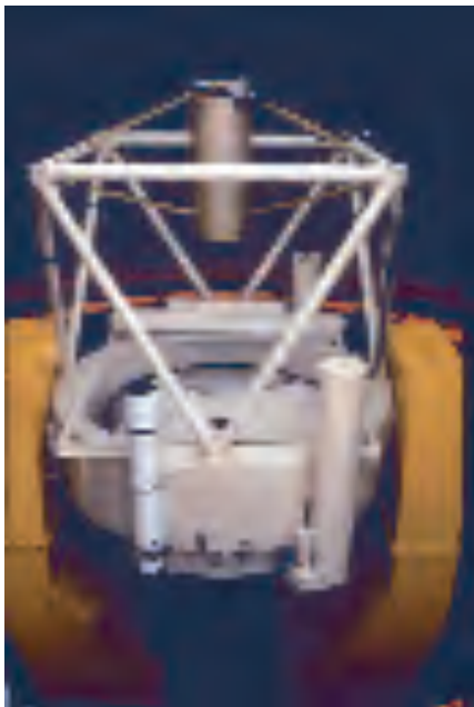
The Vatican Advanced Technology Telescope, the world's first large spin-cast mirror (1.8 meters) located at the Mount Graham International Observatory in Arizona. Photo courtesy Christopher Corbally SJ.
