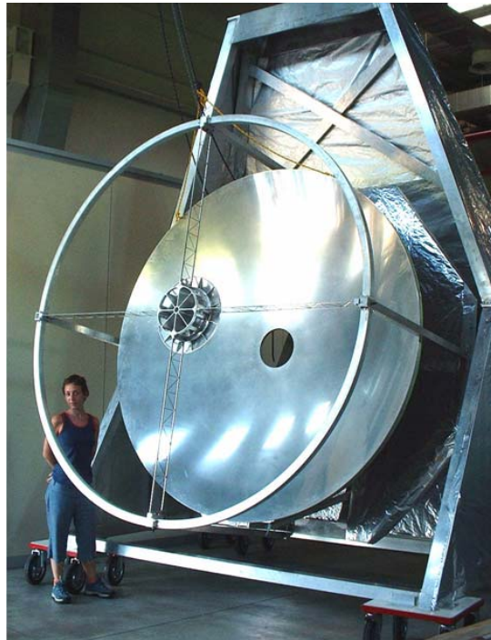
Figure 3: The OLIMPO balloon-borne telescope (the ground and sun shields are not present, revealing the 2.6m mm-wave telescope with steerable primary mirror).
