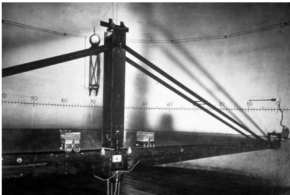
Above Proof of the Earth's rotation was derived from Fr. Hagen's "Isotomeografo", which detected the tiny Coriolis force acting on weights moving in a North-South direction. When the two weights on wheels, each massing 90 kg, moved towards the center of the device, the change in their position relative to Earth's spin would result in a slight counter-clockwise motion of the beam on which they moved, as indicated by the arrow painted on the wall.
